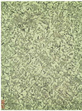
Etial 160 Aluminum Magnification: 100 x
